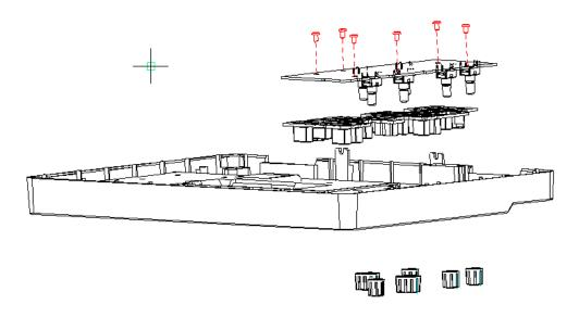
Figure 17 To remove the rubber keypad and keyboard
