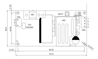
Figure 18 Power supply module mechanical drawing
