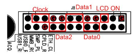
Figure 27 Test points for LCD signal
