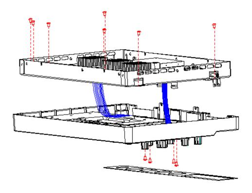
Figure 16 To remove the mainboard and front panel
