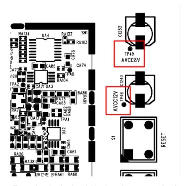
Figure 23 Test points for the Acquisition board power supplies (continued)
