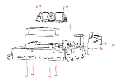
Figure 15 To remove the power supply module and fan.
