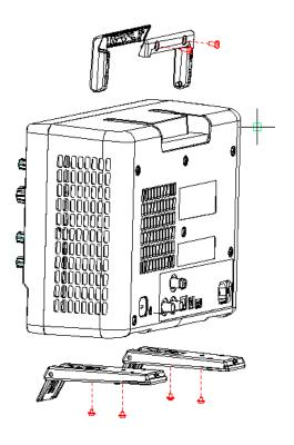
Figure 11 To remove the handle and foot
