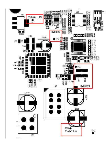
Figure 19 Test points for the Acquisition board power supplies
