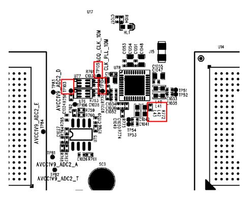
Figure 24 Test points for clock
