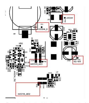
Figure 21 Test points for the Acquisition board power supplies (continued)
