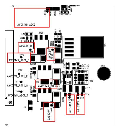
Figure 22 Test points for the Acquisition board power supplies (continued)
