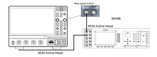
Figure 9 Test setup for Ext trigger level
