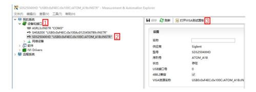
4. Click "Open VISA Test Panel" option button, and then the following Interface will appear. Next, click the "Input/Output" option button and click the "Query" option button to view the Read operation information.
