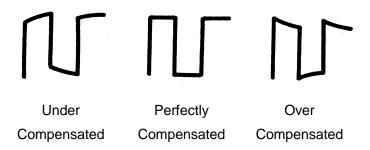
5. Use a non-metallic driver to adjust the low-frequency compensation adjustment hole on the probe until the waveform displayed is as the "Perfectly compensated" in the figure above.
