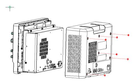
Figure 12 To remove the rear cover
