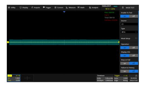
Figure 5 Mask Test Interface
