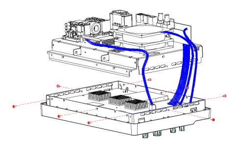
Figure 14 To remove the back panel chassis module.
