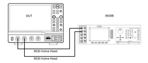
Figure 8 Test setup for Channel skew
