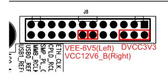
Figure 26 Test points for the LCD power supplies
